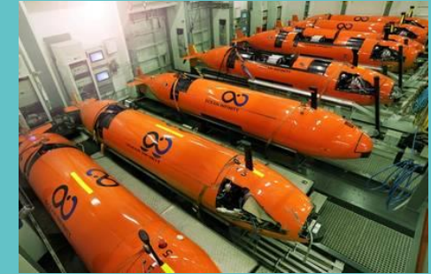
Autonomous underwater vehicle (AUV) used for high resolution seabed mapping
