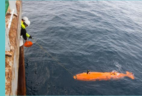
Autonomous underwater vehicle (AUV) used for high resolution seabed mapping
