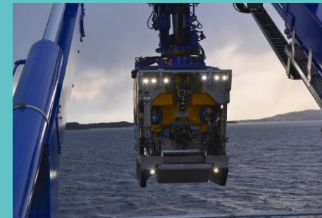
Remote operated vehicle (ROV) used for sampling and more detail mapping of the seabed
