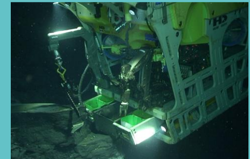
Remote operated vehicle (ROV) used for sampling and more detail mapping of the seabed
