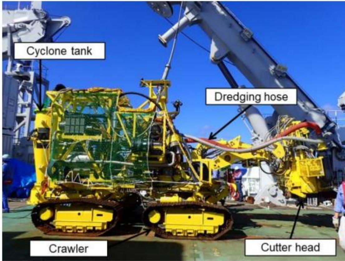
Crust-excavation testing machine
