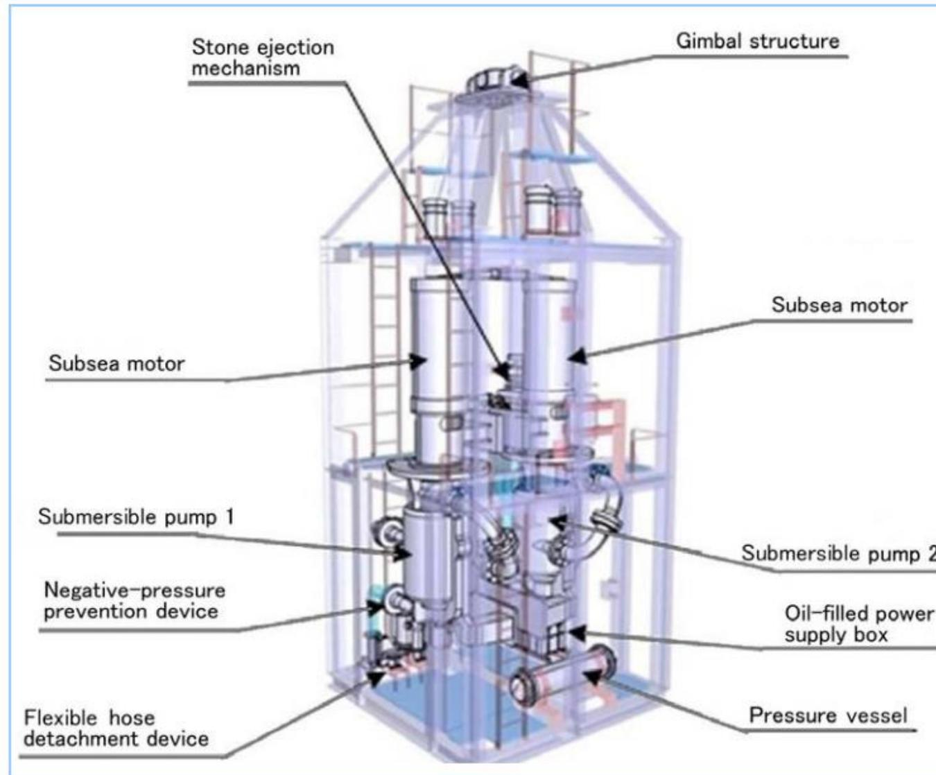
**Figure 5 Submersible pump unit configuration**
