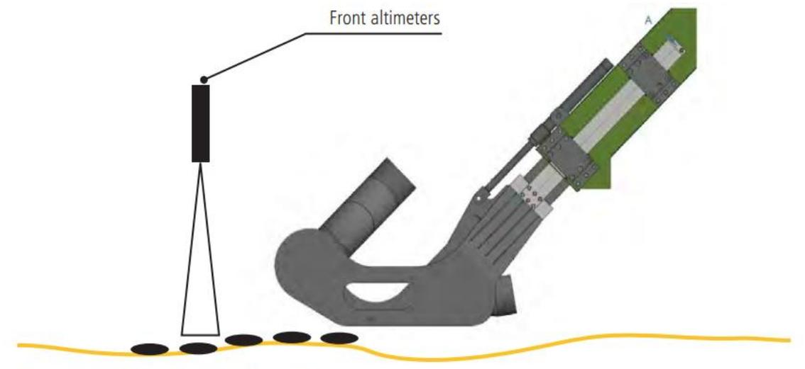
Figure 11: Collector head height control
