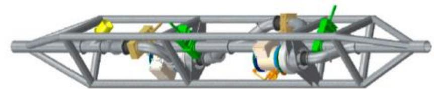
FIG. 8. MEMBER TYPE CONCEPT BOOSTER STATION FOR THE VTS, CONSISTING OF TWO CENTRIFUGAL DREDGE PUMPS AND SEVERAL VALVES.
