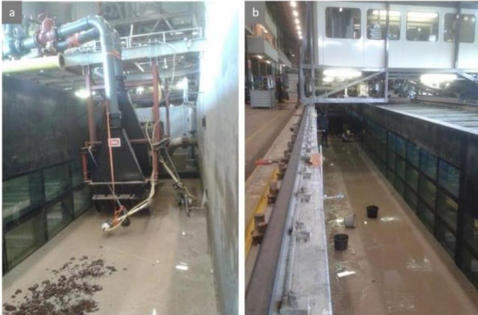
Figure 3.4. Full-scale lab testing of the hydraulic nodule collector at the Deltares test facility in Delft, The Netherlands. a: The prepared test bed, made of lava stones on fine sand, with the collector in the background; b: the test bed after the collector has passed over it. Photo Henko de Stigter.
