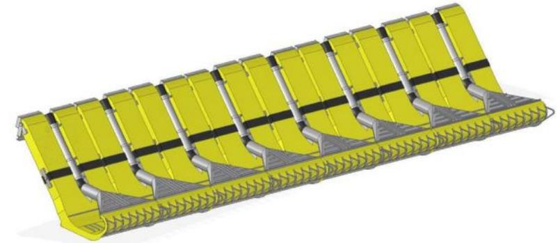
Figure 3.3. Artist impression of full-scale hydraulic collector, composed of 8 separate 2 m wide units. The pre-prototype nodule collection vehicle Apollo II is equipped with one half-scale unit. Reproduced from Blue Nodules Deliverable 2.2.
