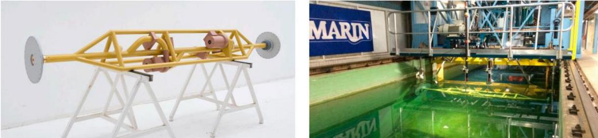
FIG. 10. SCALE 1:6 BOOSTER STATION TESTED IN THE MARIN BASIN TO FIND THE HYDRODYNAMIC COEFFICIENTS WHICH ARE NECESSARY FOR CFD MODELLING OF RISER DYNAMICS.
