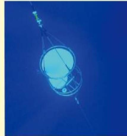
Mooring observation system with attached sediment trap
