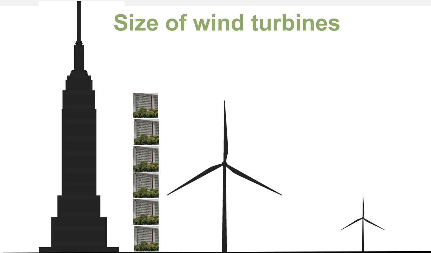
State of art turbine 15 MW – 270 m Rotor: 240 m
