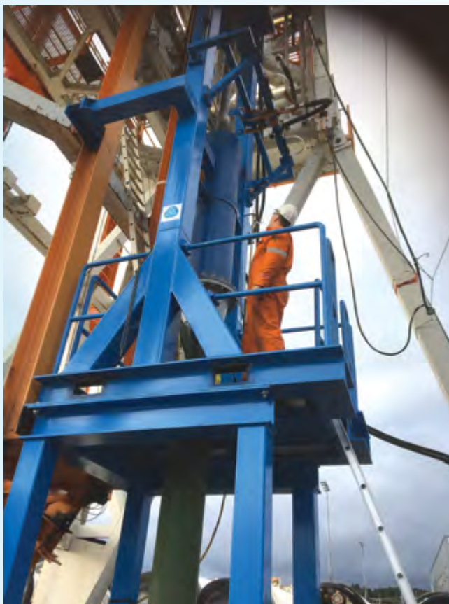
Test of RCD sealing assemblies at Mongstad, Norway 2017. Photo from ESD.
